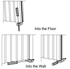
h. If the vertical rail is not aligned straight up and down, adjustment is necessary. Tighten or loosen the screw to adjust the movable rail so it is aligned straight.
