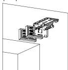
For floor bracket: Install the spacer block (1pc or 2pcs) at the backside of the Floor bracket as the next diagram shows.
