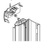
f. Press hangers onto the headrail from the front of the shade. Make sure the hangers are in the front of the middle groove in headrail.
