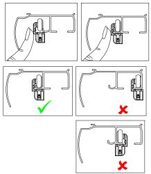
g. Attach the floor bracket to the end cap of fixed vertical rail, shown in left drawing shows.
