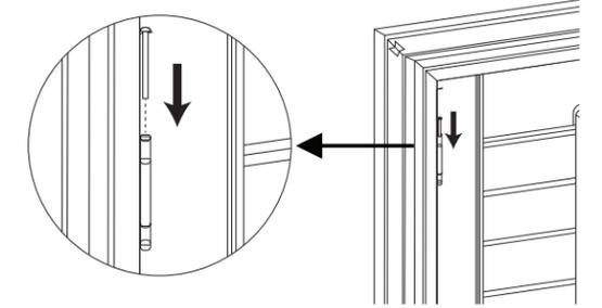
2. If panel hinges are not aligned with frame hinges properly, then frame hinges can be adjusted.
