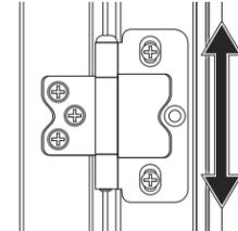
3. Please check the gap between panel and frame at the top and bottom. The gap should be even; if not, then shift frame left to right until the gap is even.
