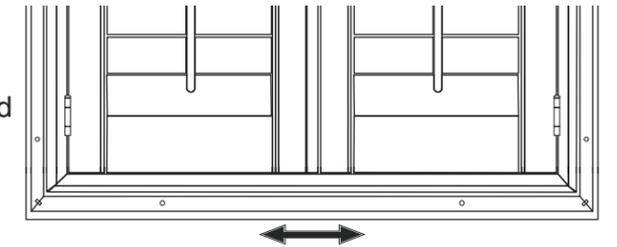
4. Once even, secure a screw at the bottom of the left frame and right frame.
