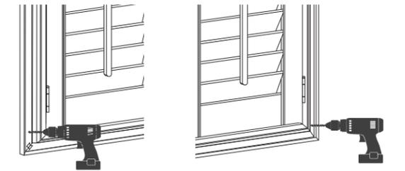
5. Open and close the panels to make sure they operate properly. Then secure the frame by tightening the rest of the screws into the frame.
