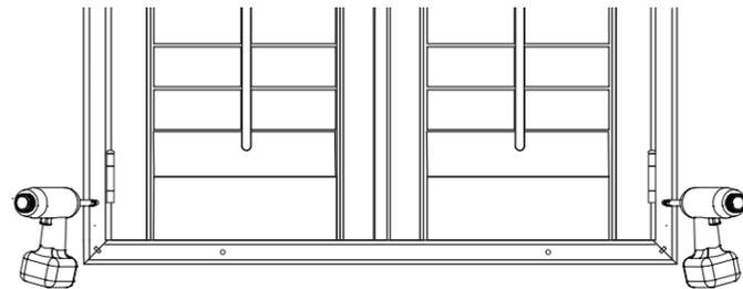
5. Open and close panels to make sure panels operate properly. Secure the frame with screws through the rest of the holes.
