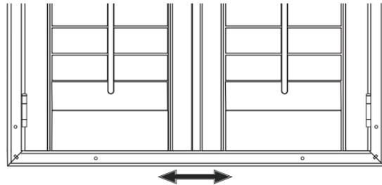
4. Once even, secure a screw at the bottom of the left frame and right frame.
