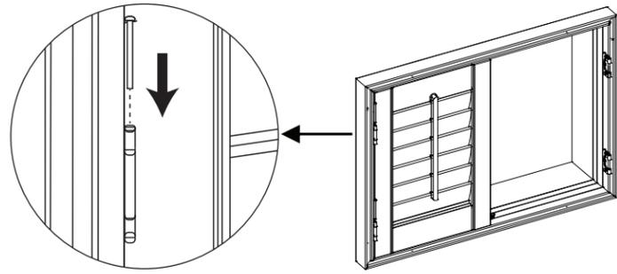
2. If panel hinges are not aligned with frame hinges properly, then frame hinges can be adjusted.
