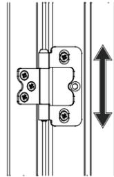
3. Please check the gap between panel and frame at the top and bottom. The gap should be even; if not, then shift frame left to right until the gap is even.
