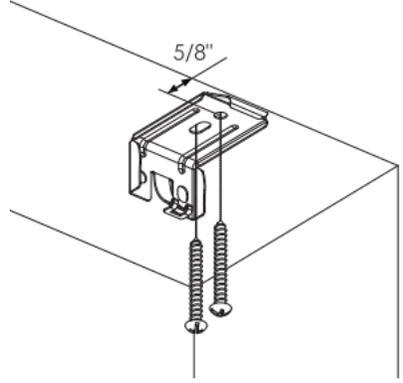
If you would like your shade to be flush with the wall, the distance from the wall to center of 1st screw hole needs to be 5/8".
