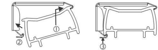
Fully raise the shade that you want to remove. Remove the shade by pushing the latch back. Release the shade by rotating the headrail towards you and lifting upward to unhook the rail from the bracket. See steps 1 to 3.
