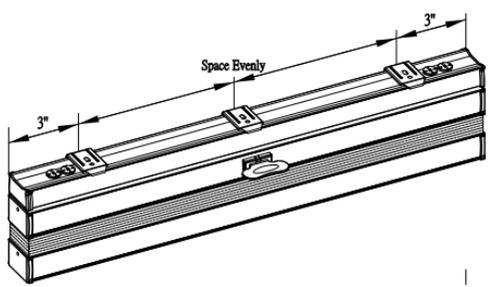
• Measure 3" from both ends of the headrail and mark the bracket location on the mounting surface (applies to both inside and outside mount installation).
