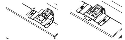
**Step 3:** If the female brackets are a little off from the male bracket, the position of the female brackets can be adjusted by moving left or right 5/16".
