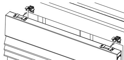
**Step 2:** Slide the female bracket on the shade into
