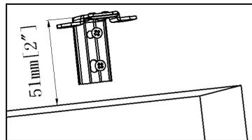
The combination of bracket and one spacer block
