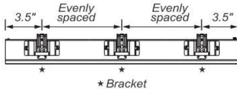
**\*\* Proper alignment of brackets will make installation easier.**
