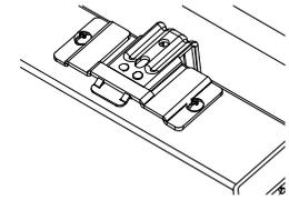
**Step 3:** If the female brackets are a little off from the male bracket, the position of the female brackets can be adjusted by moving left or right 5/16".
