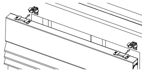
**Step 2:** Slide the female bracket on the shade into the male bracket until it snaps into place. **If more than two brackets are used, it is recommended to attach the center female bracket into the male bracket first, and then attach the female bracket at each end.**
