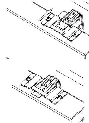
**Step 3:** If the female brackets are a little off from the male bracket, the position of the female brackets can be adjusted by moving left or right 5/16".
