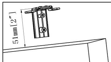
For shade width >50", the combination of bracket and one spacer block to be used. Please follow the below illustration to attach the spacer blocks, and then mount the combination of the bracket and spacer block with 2pcs 2.5" screws.
